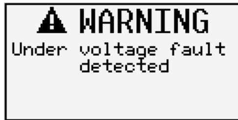
These pop-up windows can be acknowledged by pressing "OK". As long as this alarm is present, an icon is displayed in the top left-hand corner of the screen.
