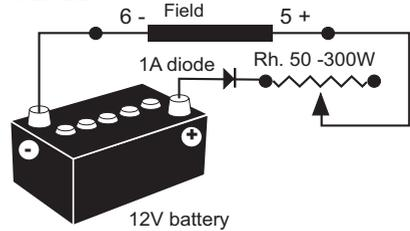
**Assembly B:** Connect a "Variac" variable power supply and a diode bridge on both exciter field wires (5+) and (6-).
