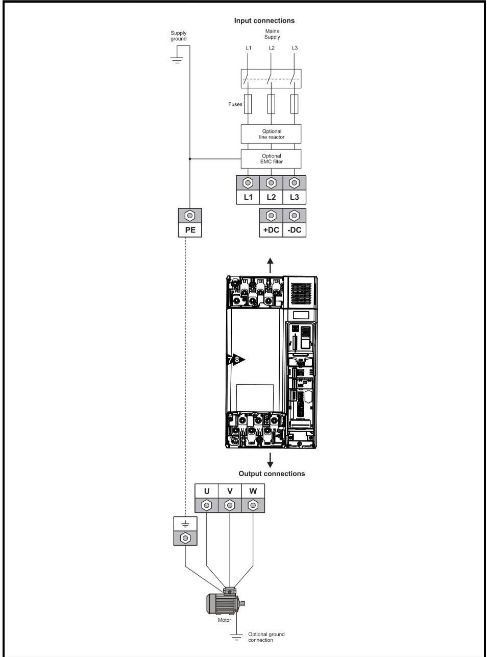
Figure 6-6 Size 9E, 10E power and ground connections
