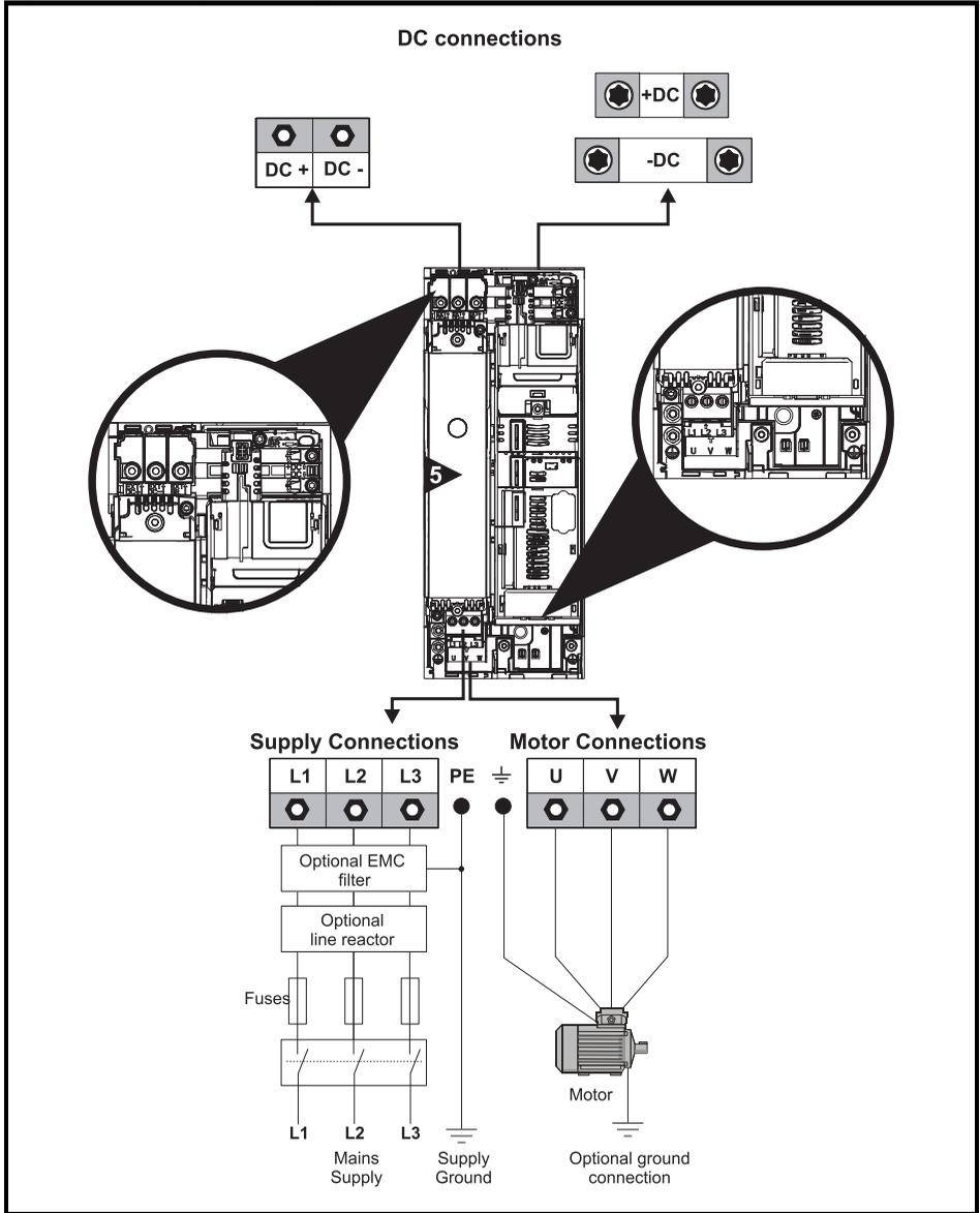
**Figure 6-4 Size 6 power and ground connections**
