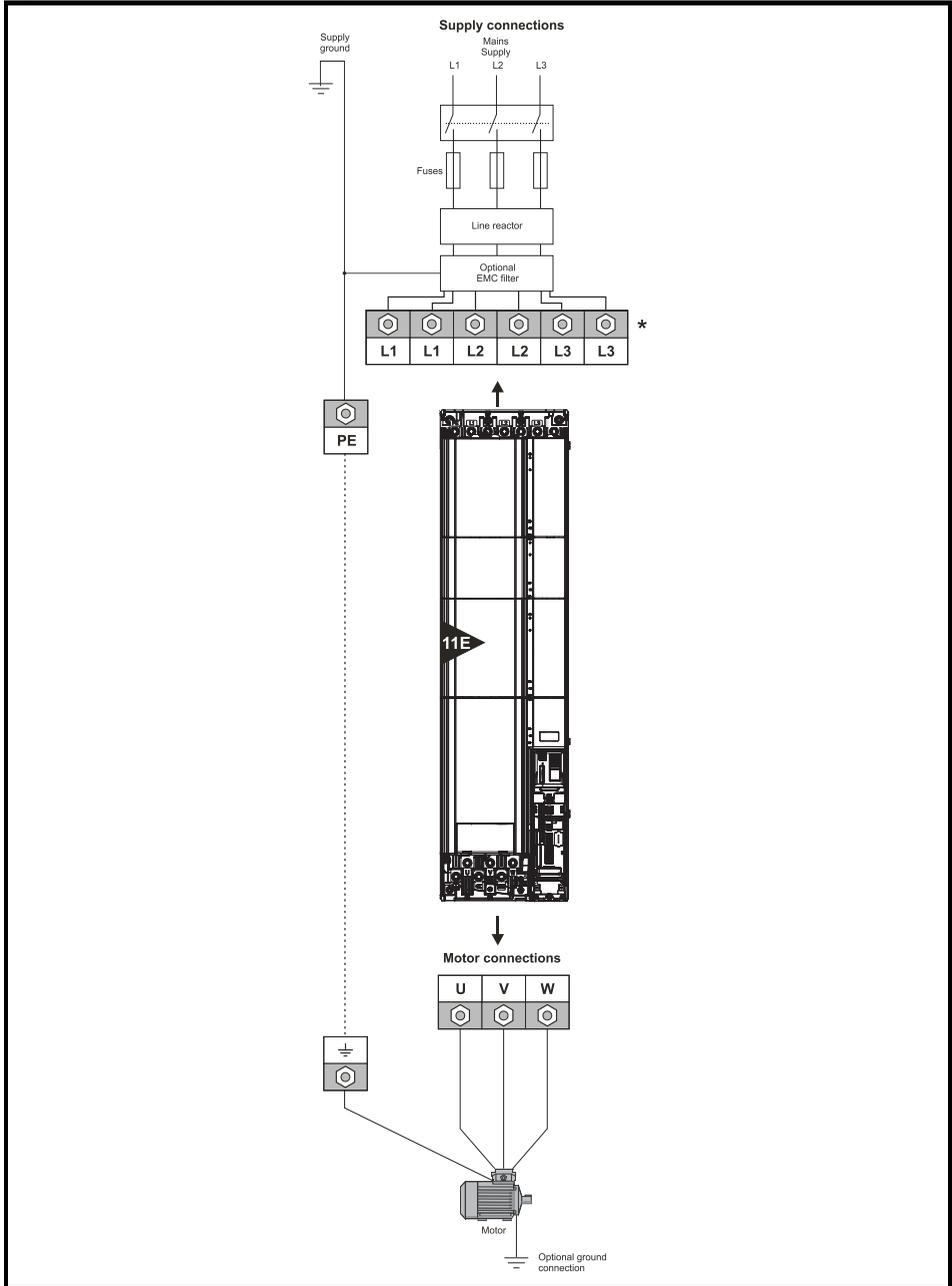
**Figure 6-9 Power Module Frame 12 power connections**
