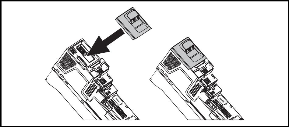
To install, align the KI-485 Adaptor and press gently in the direction shown until it clicks into position. To remove, reverse the installation instructions.
