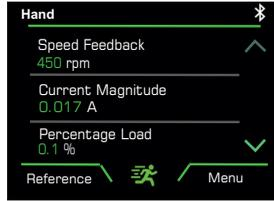
If the motor appears to be running in the wrong direction stop the drive from running by pressing the red OFF / Reset button or by opening the Hand switch. The software status changes to Off (Ready). Either reverse two motor phases electrically when safe to do so, or alternatively, set Reverse Output Phase Sequence Pr **05.042** to On.
