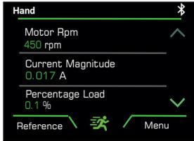
If the motor appears to be running in the wrong direction stop the drive from running. Either reverse two motor phases electrically when safe to do so, or alternatively, set Reverse Output Phase Sequence Pr **05.042** to On. To do this in software, stop the motor by pressing the red OFF / Reset button or by opening the Hand switch. The software status changes to Off (Ready).
