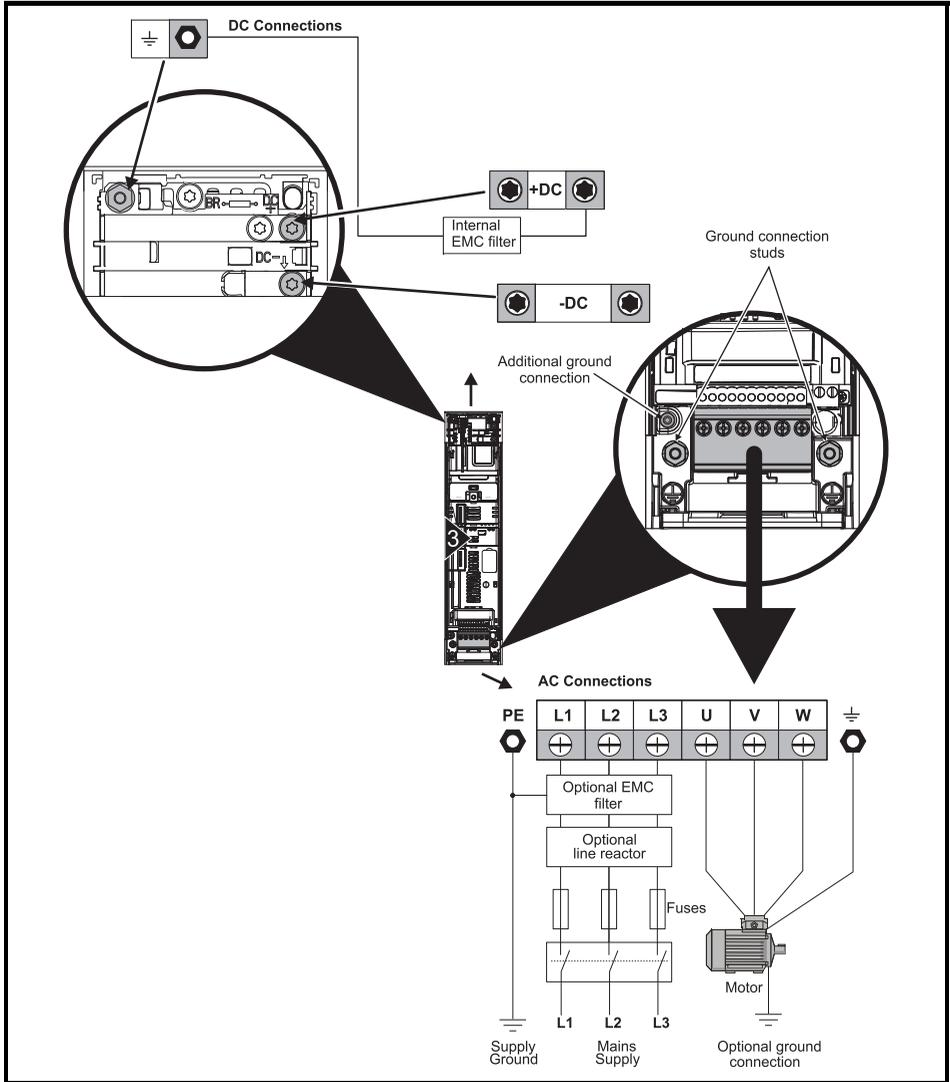
**Figure 6-2 Size 4 power and ground connections**
