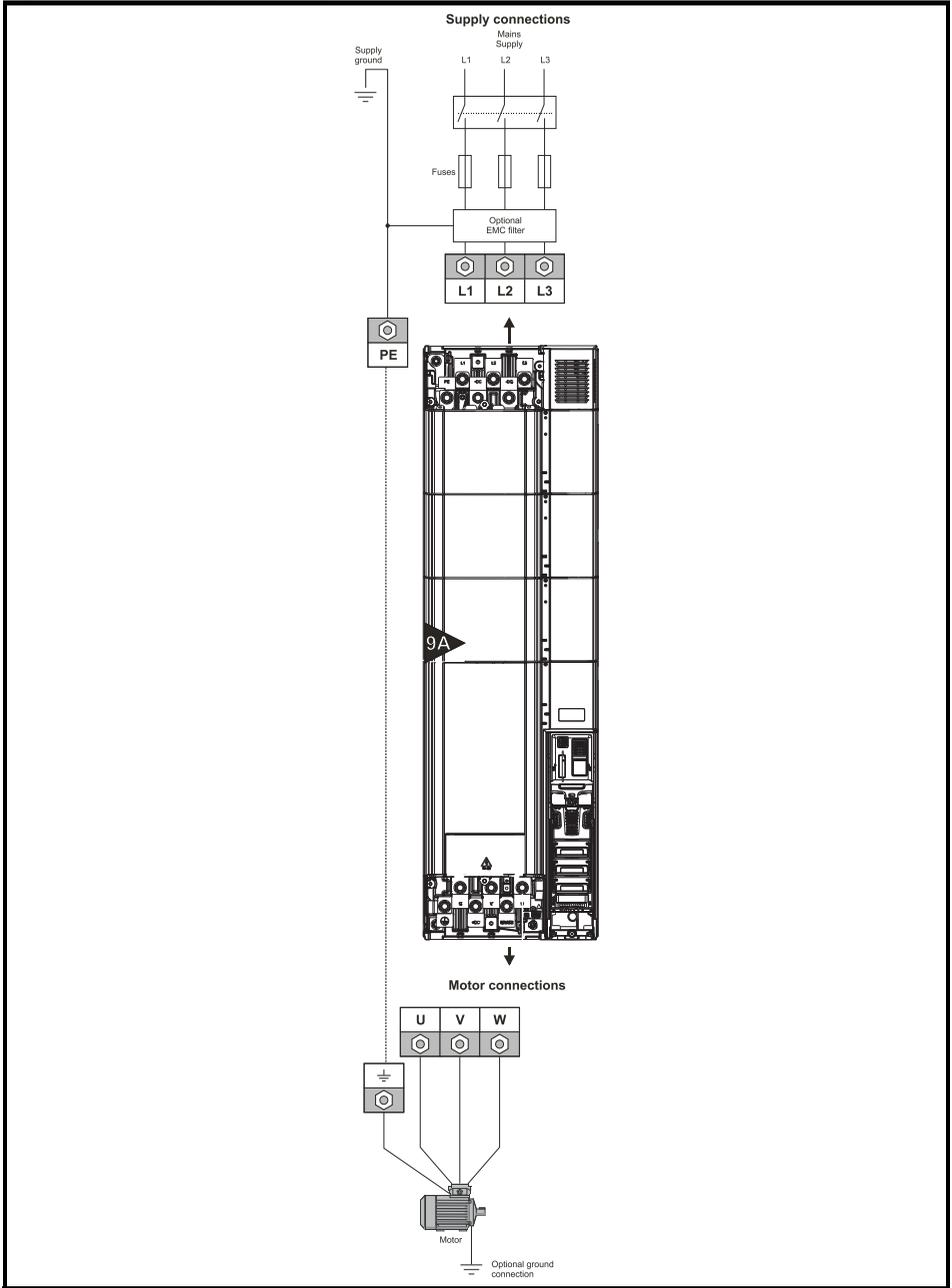
**Figure 6-8 Size 11E power and ground connections**
