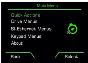
Use search facility to then access a known parameter value, by selecting the actual value using the Navigation Up/Down Left /Right keys. Use select to move to next screen, to change the parameter setting select edit and then use the navigation keys to select the number field.
