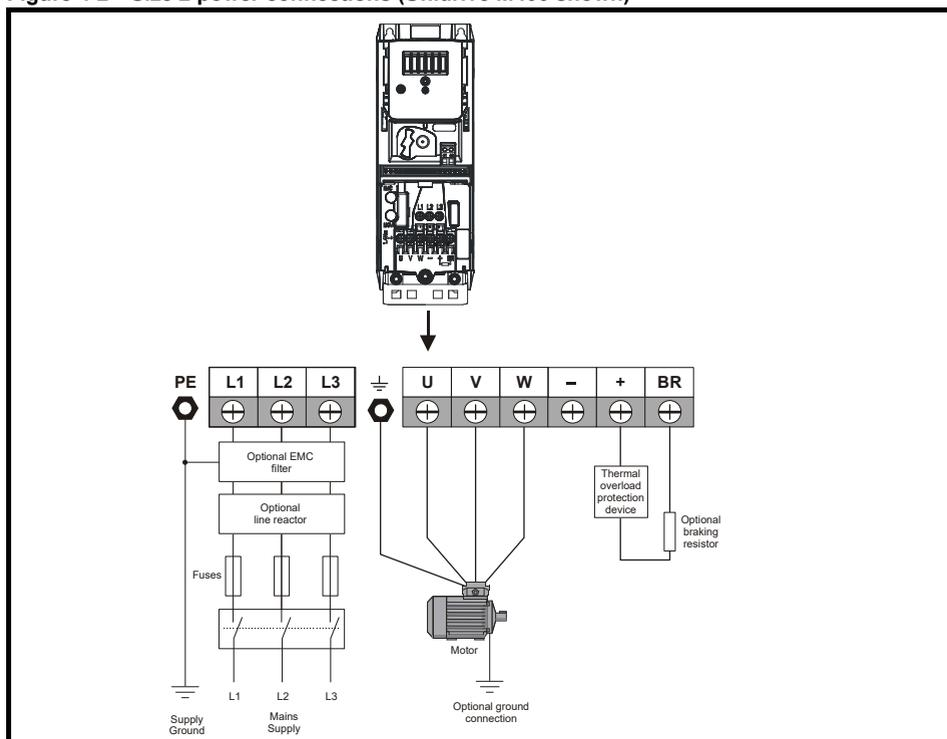
See Figure 4-5 *Size 1 to 4 ground connections (Unidrive M400 size 2 shown)* on page 46 for further information on ground connections.
