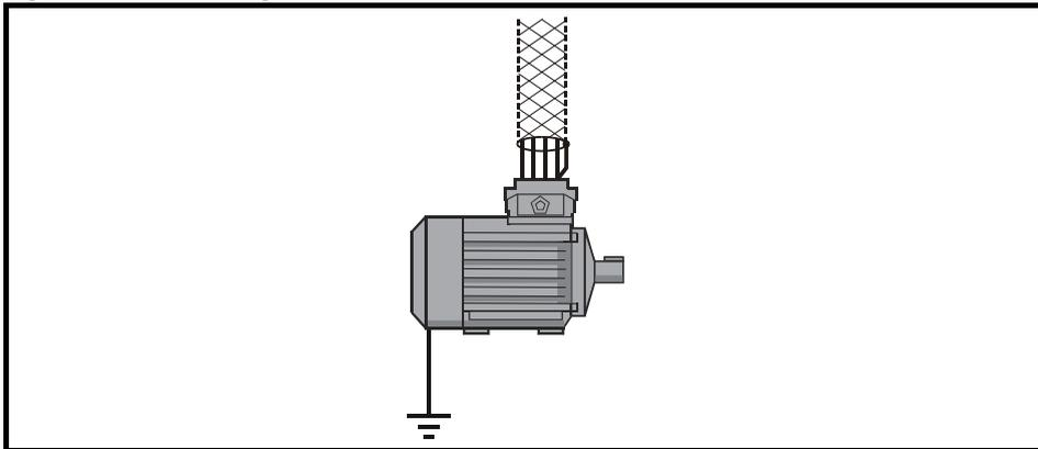
Unshielded wiring to the optional braking resistor(s) may be used provided the wiring runs internally to the enclosure. Ensure a minimum spacing of 300 mm (12 in) from the signal wiring and the AC supply wiring to the external EMC filter. If this condition cannot be met then the wiring must be shielded.
