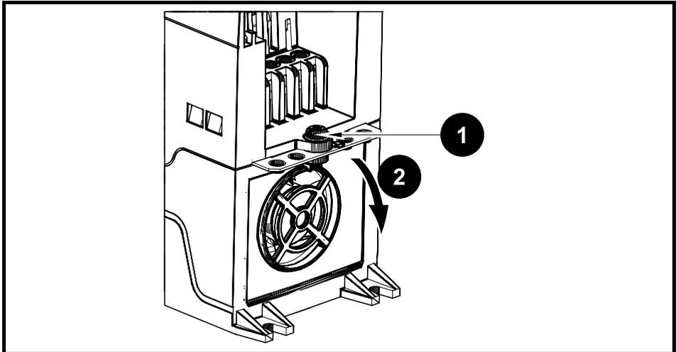
1. Remove the screw from the drive (size 1: Torx 10, size 2 to 4: Torx 20).
