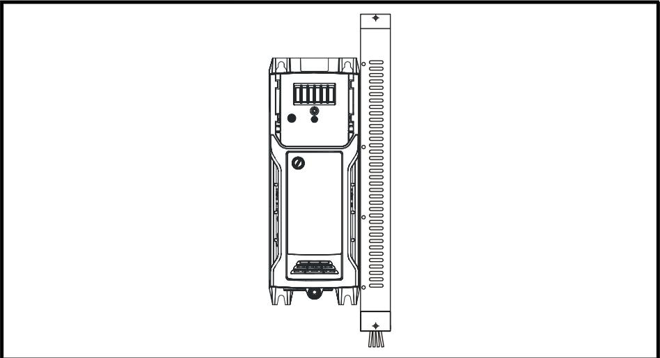
**Figure 3-11 Size 1 to 4 external EMC filter**
