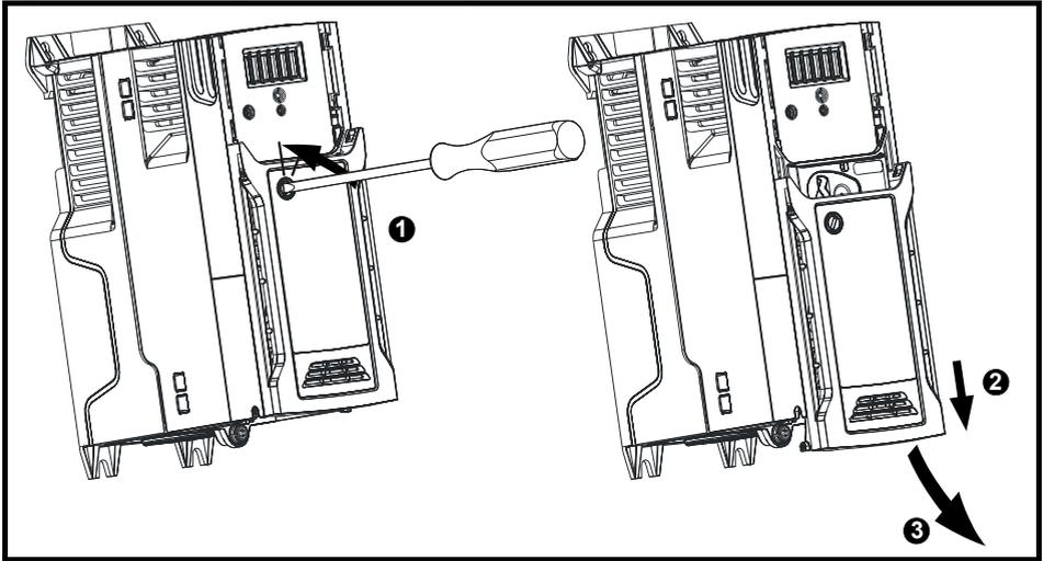
1. Using a flat bladed screwdriver, turn the terminal cover locking clip anti-clockwise by approximately 30°
