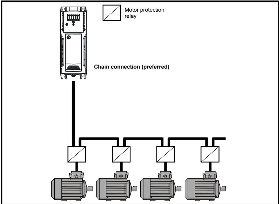
Figure 4-10 Alternative connection for multiple motors
