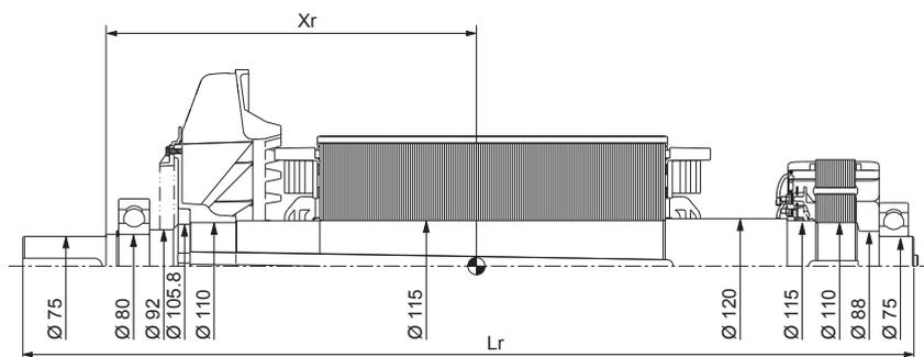
Centre of gravity: Xr (mm), Rotor length: Lr (mm), Weight: M (kg), Moment of inertia: J (kgm<sup>2</sup>): (4J = MD<sup>2</sup>)
